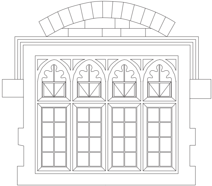
Proposed condition of window to Tower Bridge Arch 02 with reinstated glazing and frames and restored stonework tracery - exterior view
